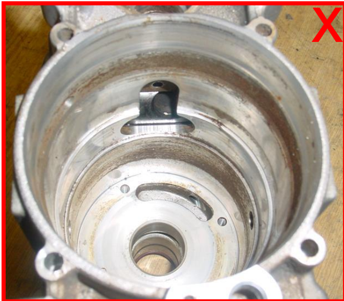
corrosion in interior-space → not acceptable
