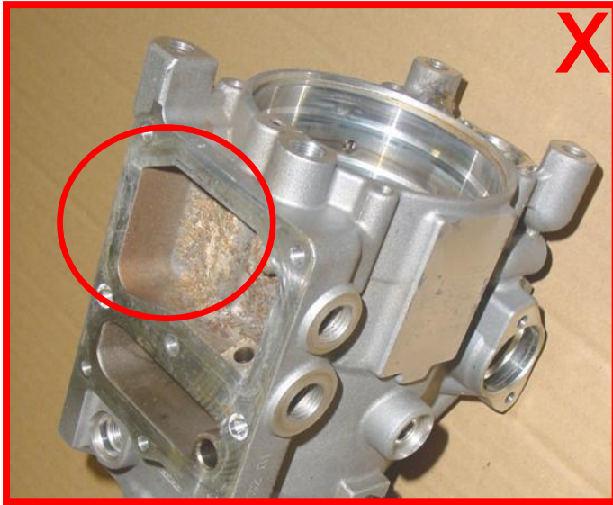
corrosion on PSG-face → not acceptable
