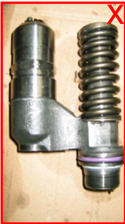
nozzle missing → not acceptable
