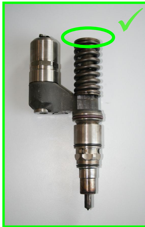
plug missing on spring plate → acceptable
