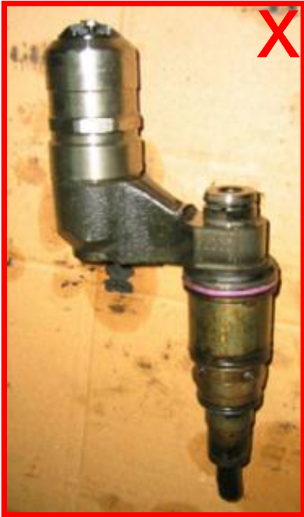
spring plate missing → not acceptable
