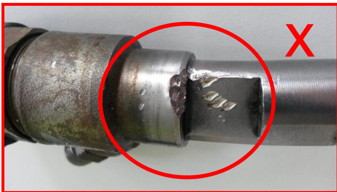
Damage on body caused by inappropriate handling (e.g. hammer) → not acceptable
